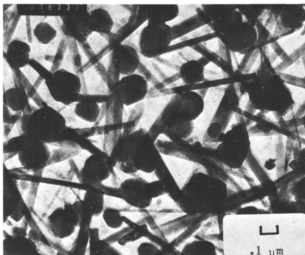
Figure 3. Spheres and rods in Lower Kittanning vitrinite shown after cooling on the heating stage of the TEM.
